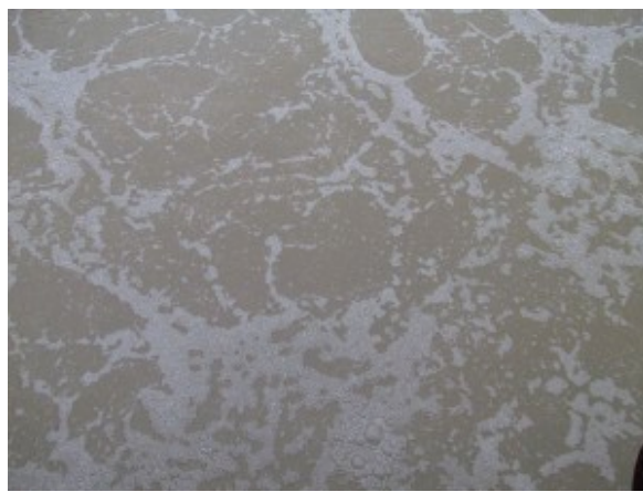
Activated sludge at the sewer plant.
