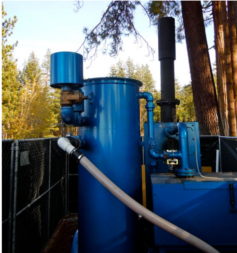
A sparge unit injects air into the soil to get the vapors out. Photo/LTN file
