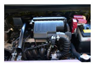
**Specifications** Engine 1193 cc DOHC 12 valve inline three cylinder 78 hp @ 6,000 74 lb.-ft. of torque @ 4,000 Transmission Five speed manual CVT automatic Configuration Transverse front engine/front wheel drive Dimensions Wheelbase 96.5 inches Length 149.4 inches Width 65.6 inches
